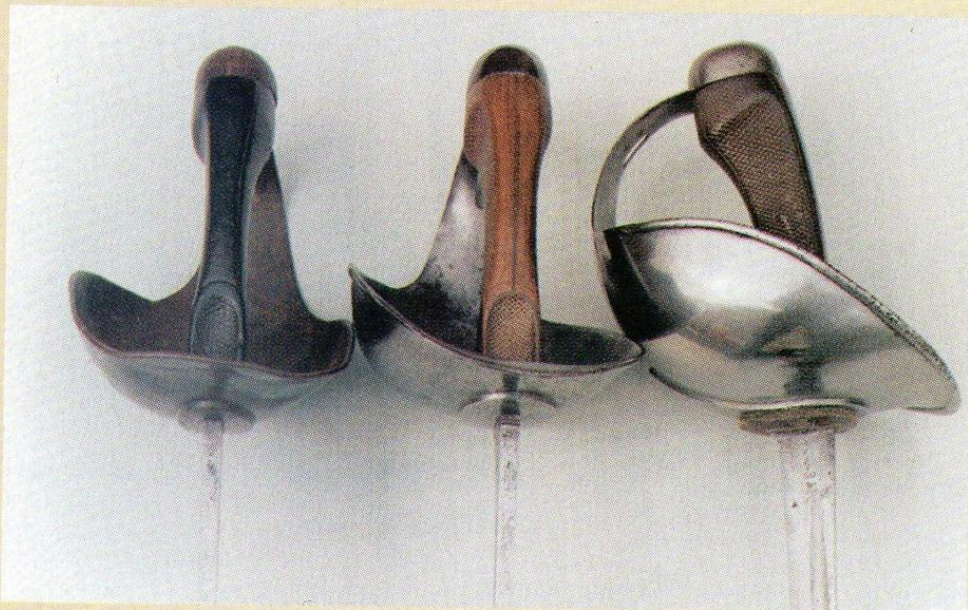
Fig. 11. Close up of hilts. The left hand sword is a MK1 with no provision for securing the buff washer, note also the narrow 1 and 1/4 ins. wide mullet. The centre sword is also a MK1 but has the serrations to back and front of blade to hold the washer in place; note the wider mullet introduced in August 1910. The right hand No.1, MK1* sword has the pin through the blade to hold the washer firmly against the hilt; LoC. 16089, May 1912.
